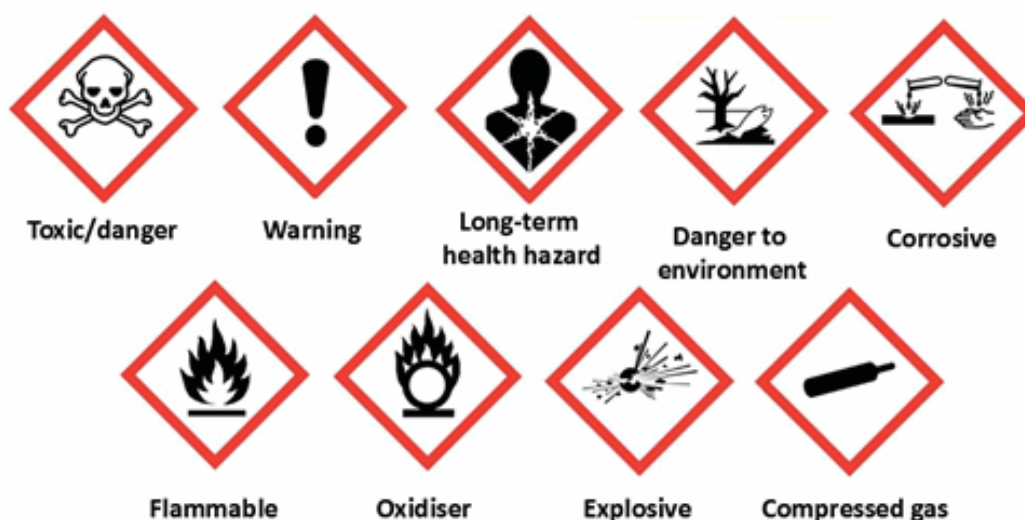
Fig. 1: Common hazardous substance symbols
