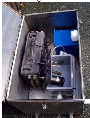
Figure 3.3 The prototype Automatic River Monitoring Station (ARMS).
