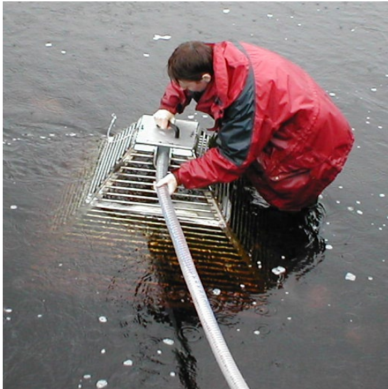
Figure 3.1 The variant of the Automatic River Monitoring Station deployed in the Glenamong. This uses an in situ system of sensors mounted in a strong protective cage.
