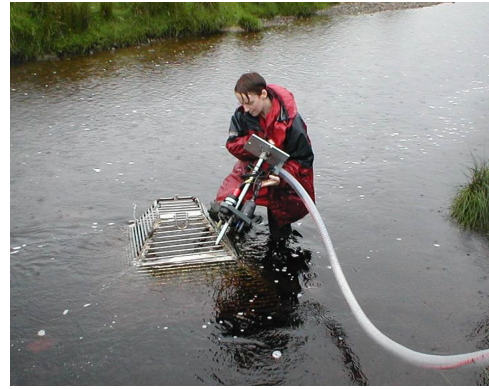
Figure 3.6 The variant of the Automatic River Monitoring Station using an in situ system of sensors mounted in a strong protective cage
