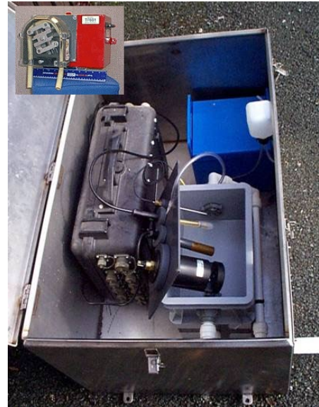
Figure 3.2 The variant of the Automatic River Monitoring Station deployed in the Rough and Black Rivers. This uses a mains-powered peristaltic pump (inset) to deliver water to a system of sensors mounted in a flow cell.
