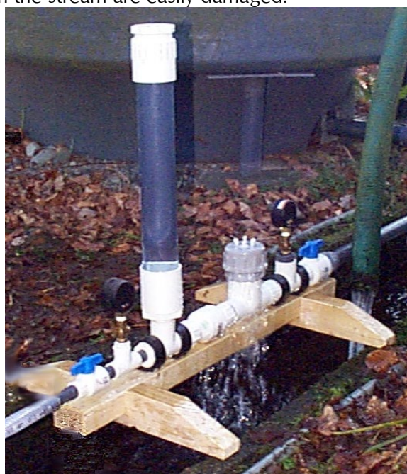
Figure 3.4 The hydraulic ram pump used on the original prototype
