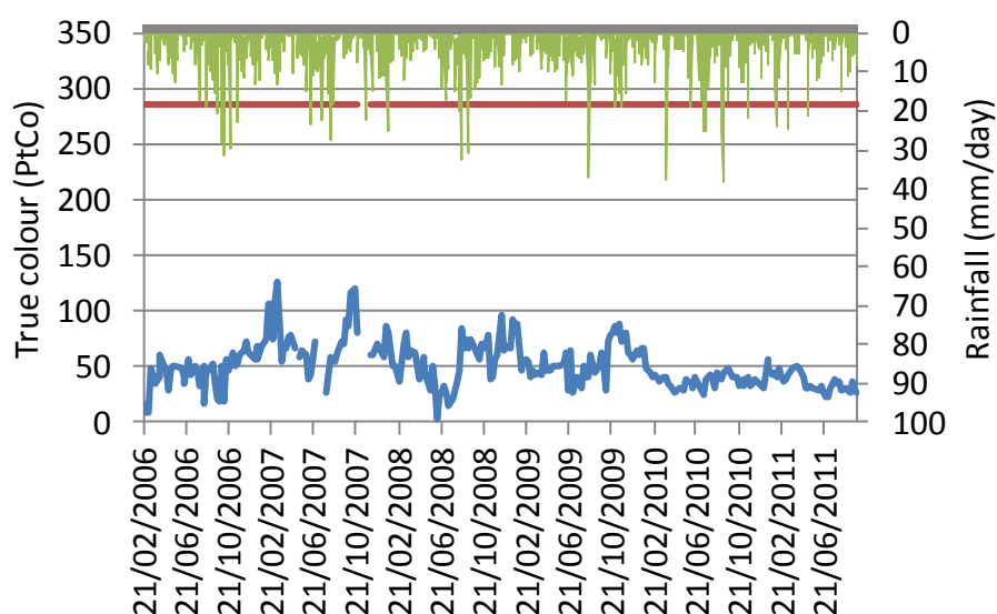
Figure 9. Raw water true colour from Drumkeery Lough (based on Veolia Water data). Red line represents the max allowable value for true colour based on the design contract (primary axis). Green bars represent daily rainfall at the Armagh Observatory.
