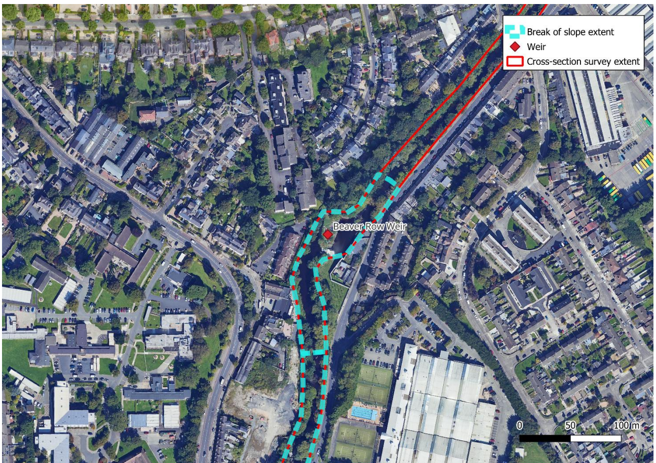
Figure 4-9 Further detail of Break-of-Slope survey extent near the Beaver Row Weir
