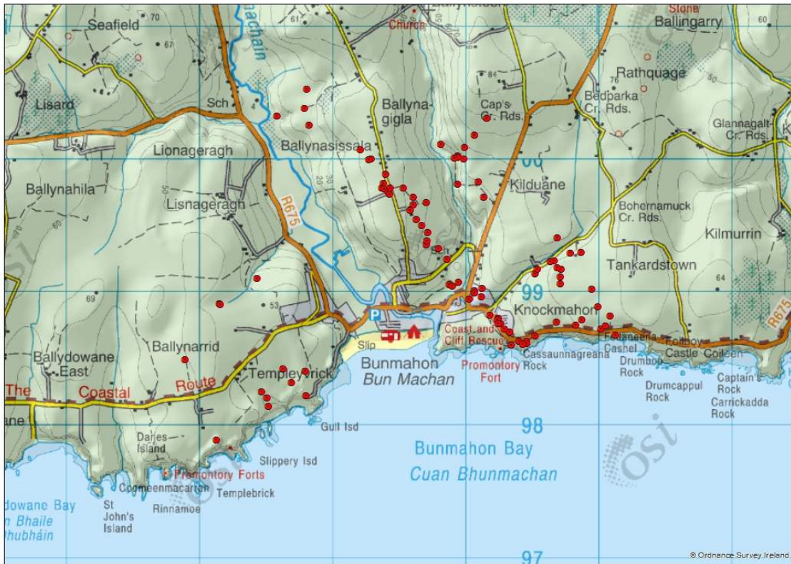
Figure 2 Approximate locations of known shaft/adit mine features at Bunmahon, Co. Waterford.
