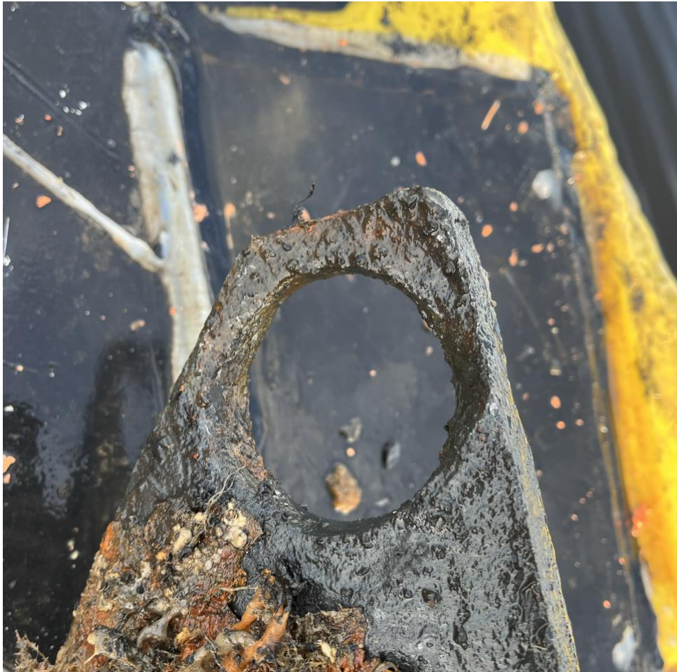
Figure 5 And 6 angel weight plate and evidence of elongation
