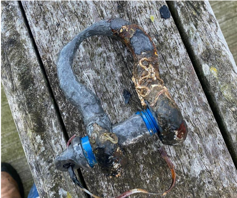
Figure 4 Example of 6.5t shackle with 90% depletion i
