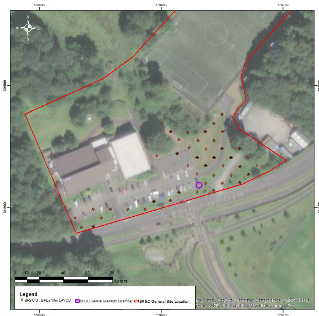
Figure A.18. SRSC geothermal collector layout
